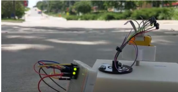
Figure 3.13 Only lidar data registered during stationary test is a false positive of the road divider: visual (left) and data model (right)
