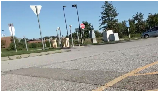
Figure 3.21 Leaning while turning the e-bike causes a false-positive result: visual camera (left) and lidar modeling (right)
