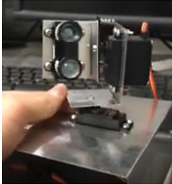
Figure 1.1 Configuration I illustrating the LIDAR-Lite v3 rangefinder and the two Towerpro servos on a bent aluminum base
